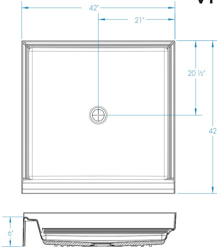
**FEATURES** Dimensional Tolerance  $\pm \frac{3}{16}$ ". Dimensions needed for site preparation should be measured from the unit. Manufacturer assumes no responsibility for preparatory work.
