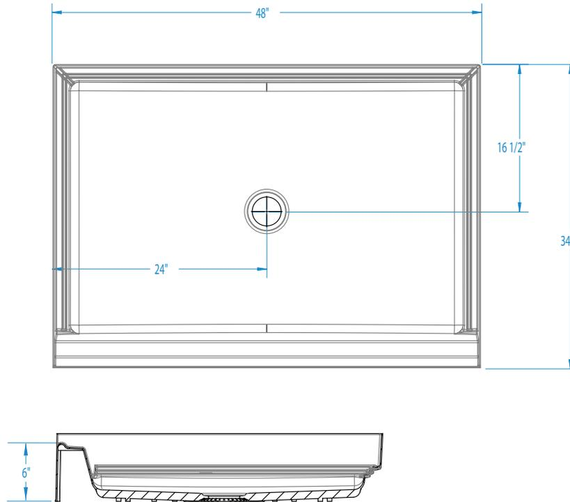
**FEATURES** Dimensional Tolerance  $\pm 3/8$ ". Dimensions needed for site preparation should be measured from the unit. Manufacturer assumes no responsibility for preparatory work.
