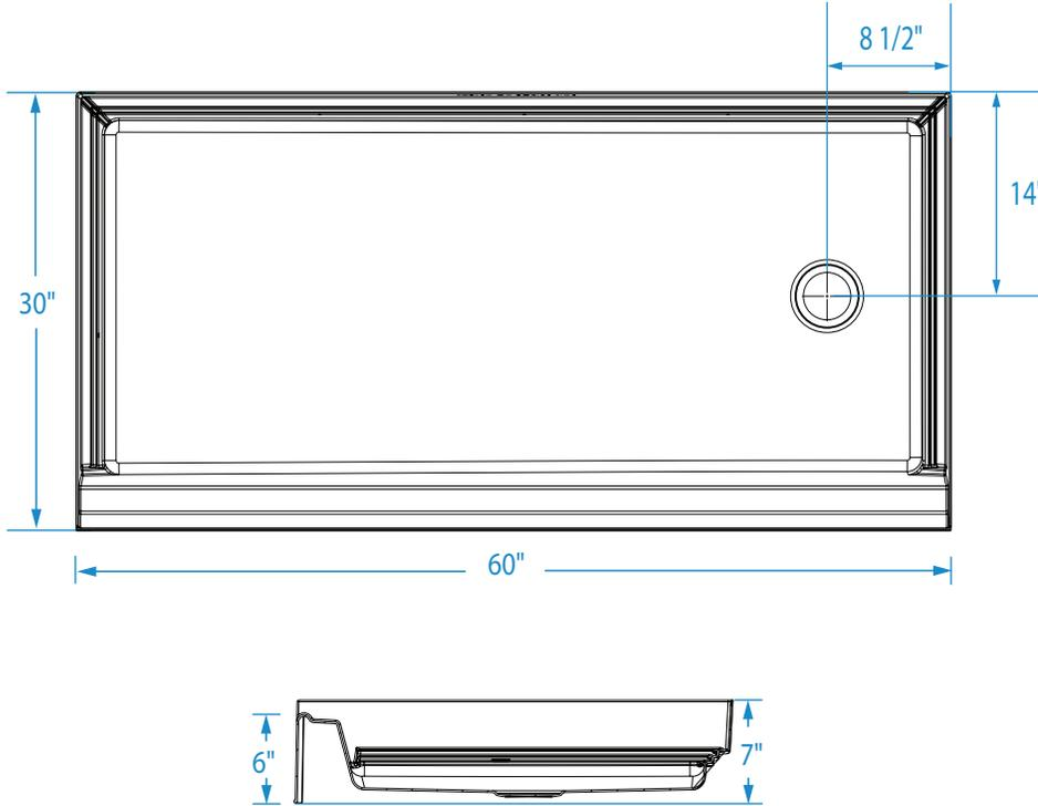
**FEATURES** Dimensional Tolerance  $\pm 3/8"$ . Dimensions needed for site preparation should be measured from the unit. Manufacturer assumes no responsibility for preparatory work.
