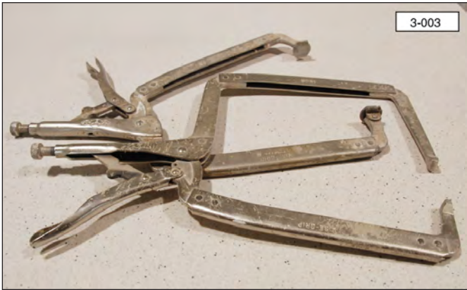
Deep throat locking plier clamps (such as Vise Grip DR18 Locking Clamp).
