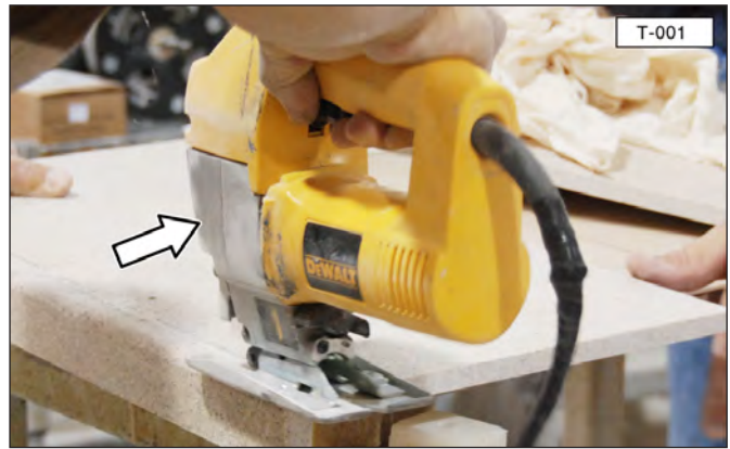
Saber saw (such as DeWalt DW317K Variable-Speed Orbital Action Saber Saw).
