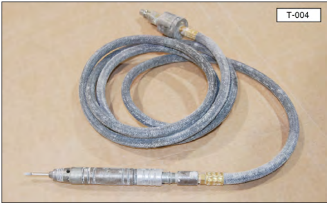
Rotary tool (such as Dremel tool or pneumatic rotary drill).
