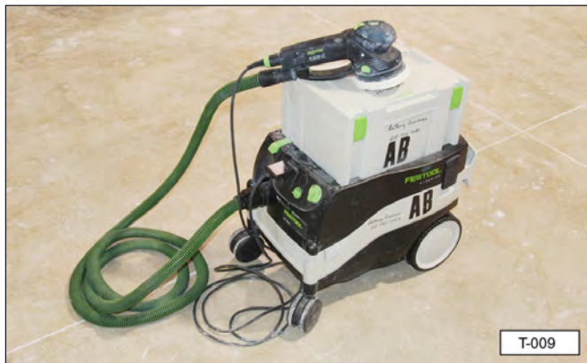
Electric sander with vacuum dust extractor (such as Festool CleanTec CT22E and RO 125 FEQ Rotex Sander).
