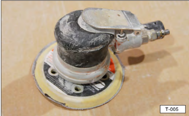
Orbital sander (such as Dynabug pneumatic sander).
