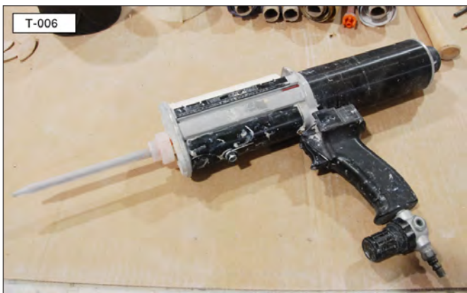
Swan Part # VW 0080.000, MixPac Type DP200-70 Pneumatic Glue Dispenser.
