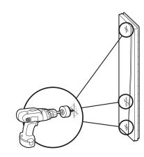
Using a hole saw (fine tooth or abrasive grit cutting edge), make necessary openings for filler and valves, drilling from inside (smooth side) out.
