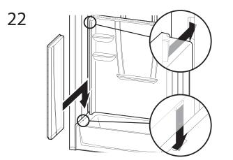
Slide left side wall into position. Be sure locking mechanism is engaged.
