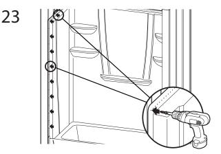
Fasten flanges along top of left side walls with fasteners of choice (see Pre-Installation Planning #12) into each corresponding stud. Fasten side (vertical) flanges to side studs 8" (200mm) on center. **NOTE:** Finish caulking is not required, however, if using caulk, weep channel must be remain clear of obstruction to allow for proper drainage of the unit.
