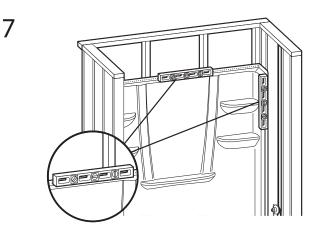
Level back wall vertically. Shim if necessary.
