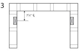
Additional stud may be required for vertical back wall flange. Stud @ 7 7/8" CL from back, on both sides. Stud can be turned for easier installation.
