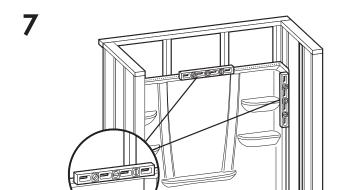
Level back wall vertically. Shim if necessary.
