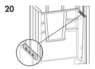
Check for level. Shim if necessary.
