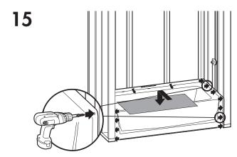
Pre-drill horizontal flanges along top of base section and fasten into each corresponding stud. Pre-drill both (vertical) side flanges and fasten to side studs 8" (200mm) on center. Place cardboard to protect surface.
