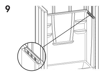
Check for level. Shim if necessary.
