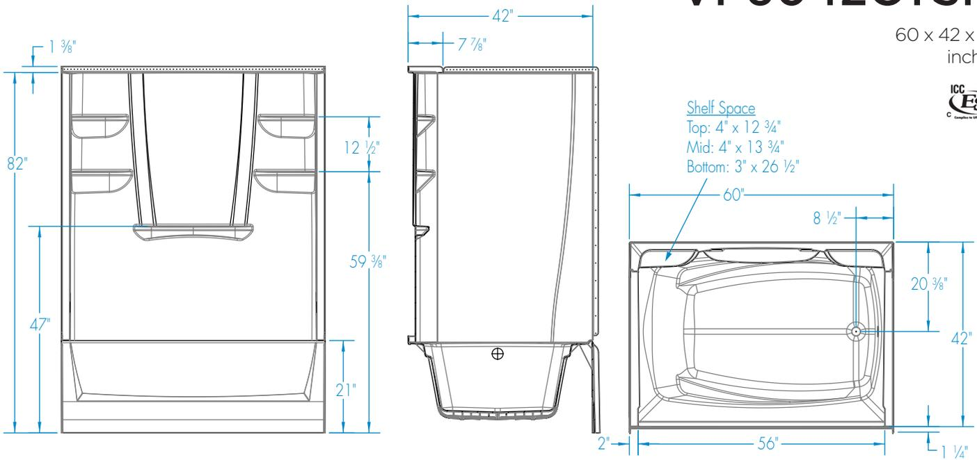
**FEATURES** Dimensional Tolerance  $\pm 3/8"$ . Dimensions needed for site preparation should be measured from the unit. Manufacturer assumes no responsibility for preparatory work.
