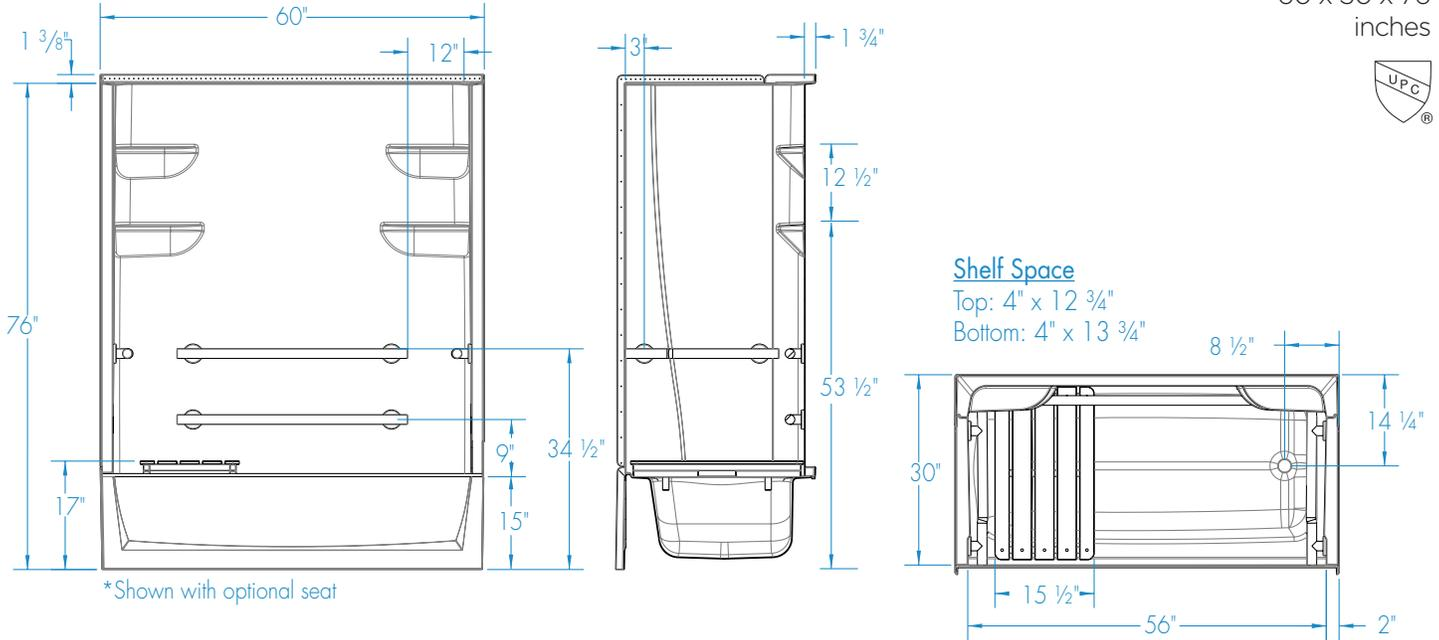
**FEATURES** Dimensional Tolerance  $\pm 3/8"$ . Dimensions needed for site preparation should be measured from the unit. Manufacturer assumes no responsibility for preparatory work.
