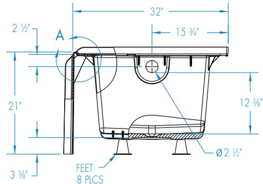
**FEATURES** Dimensional Tolerance  $\pm 3/16"$ . Dimensions needed for site preparation should be measured from the unit. Manufacturer assumes no responsibility for preparatory work.
