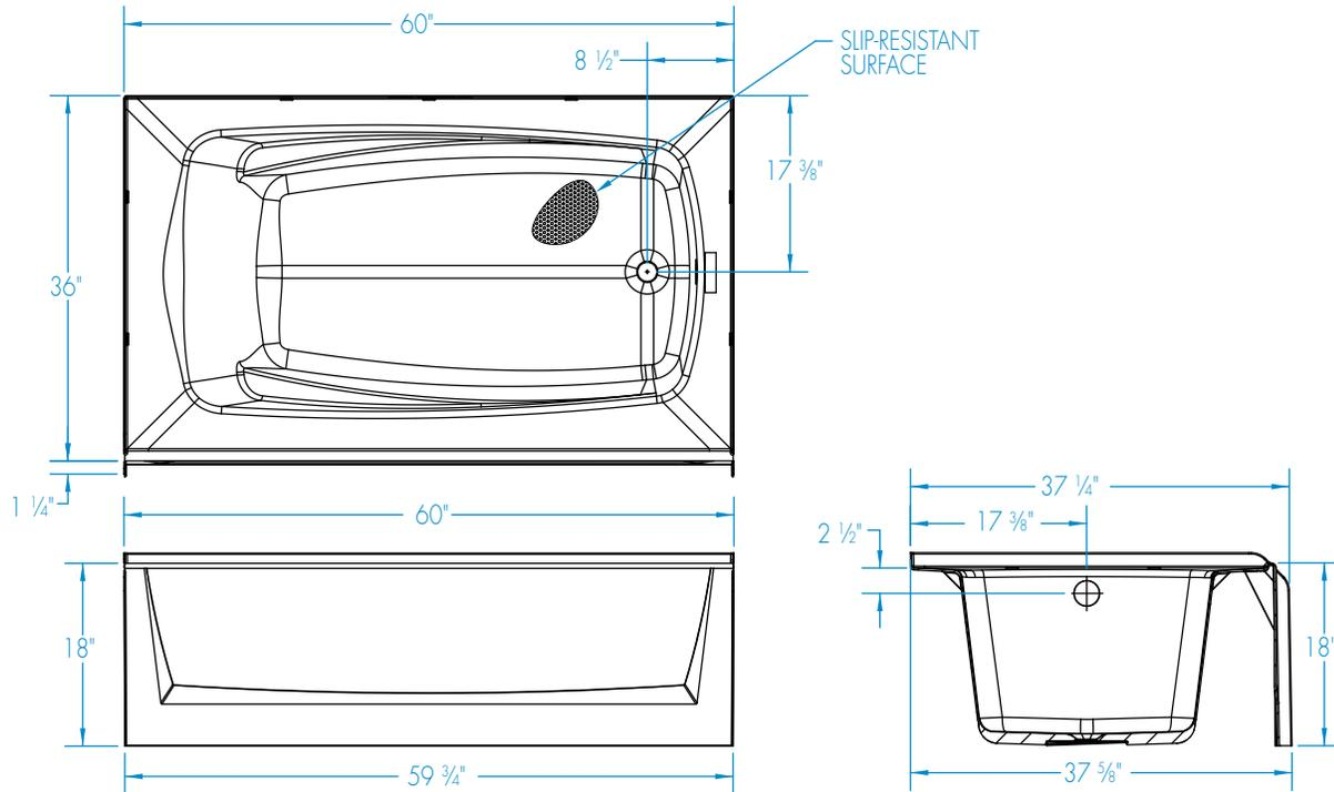
**FEATURES** Dimensional Tolerance  $\pm 3/16"$ . Dimensions needed for site preparation should be measured from the unit. Manufacturer assumes no responsibility for preparatory work.
