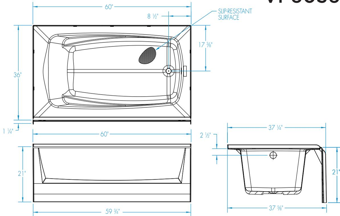
**FEATURES** Dimensional Tolerance  $\pm 3/8$ ". Dimensions needed for site preparation should be measured from the unit. Manufacturer assumes no responsibility for preparatory work.
