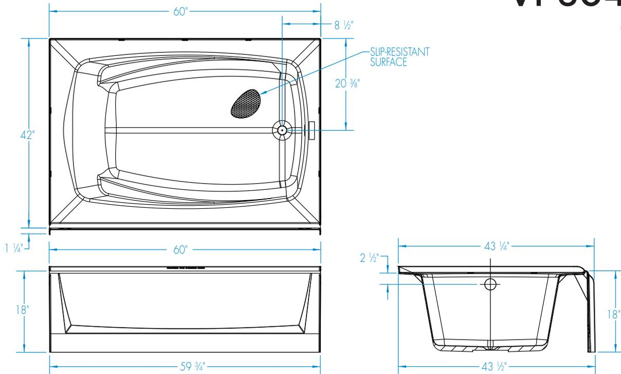
**FEATURES** Dimensional Tolerance  $\pm \frac{3}{8}$ ". Dimensions needed for site preparation should be measured from the unit. Manufacturer assumes no responsibility for preparatory work.
