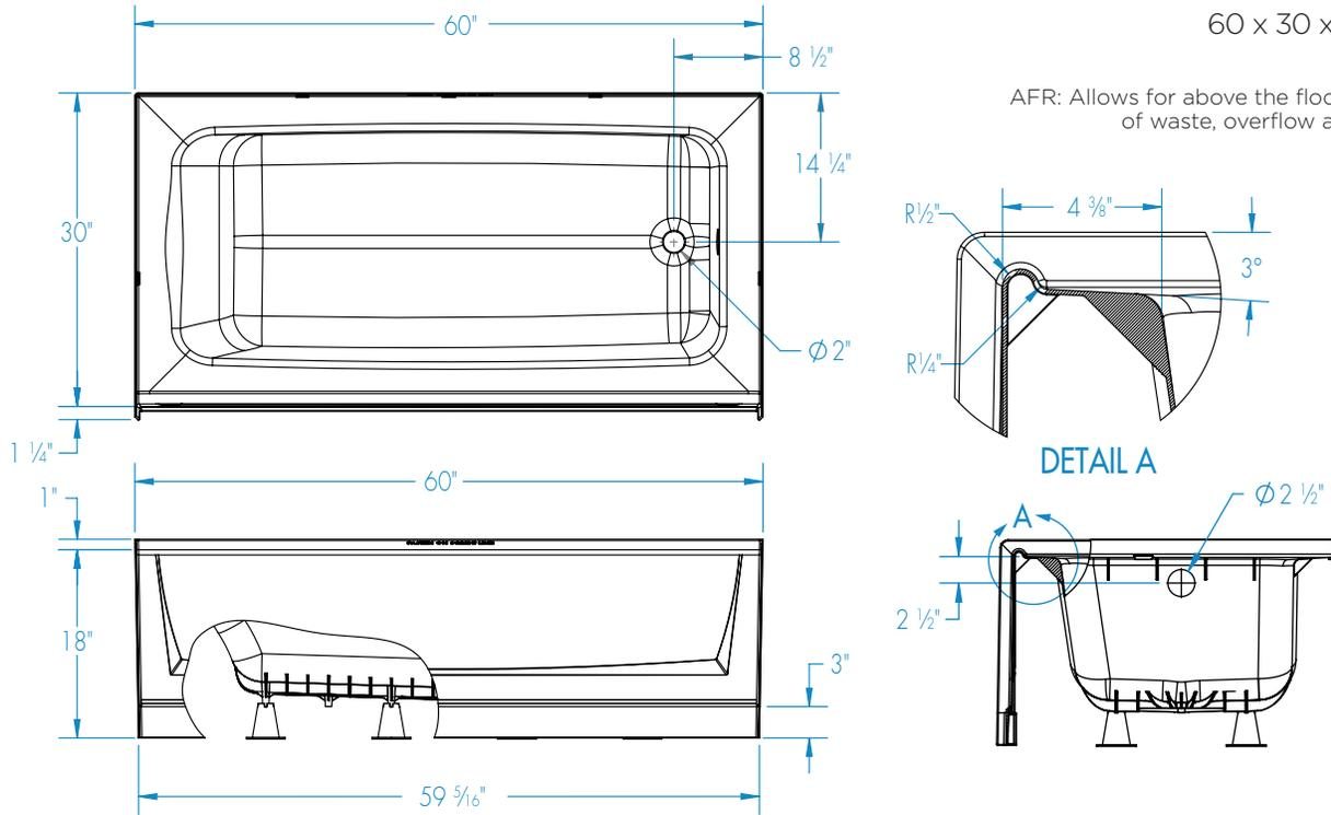
**FEATURES** Dimensional Tolerance  $\pm 3/8"$ . Dimensions needed for site preparation should be measured from the unit. Manufacturer assumes no responsibility for preparatory work.
