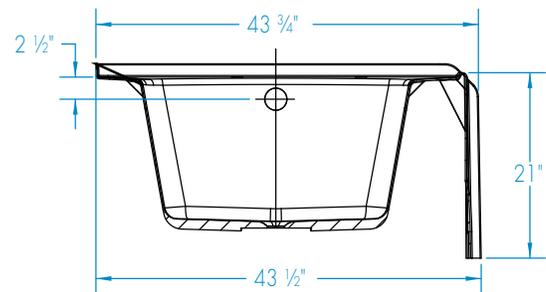
**FEATURES** Dimensional Tolerance  $\pm 3/8"$ . Dimensions needed for site preparation should be measured from the unit. Manufacturer assumes no responsibility for preparatory work.
