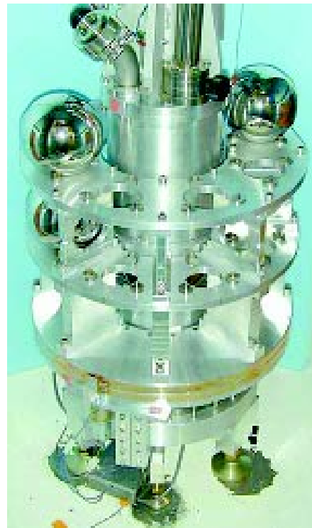
At left: The apparatus used by the research group at the University of Washington, Seattle, to measure G to record high precision. The device, about two feet across, measures the attraction between a hanging plate (hidden inside the cylinder) and several spheres which rotate about the cylinder.
