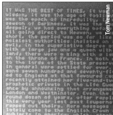
Tom Newman used an electron beam to etch the opening of Dickens' Tale of Two Cities onto a 200 x 200 micron square of plastic and won the Feynman challenge.
