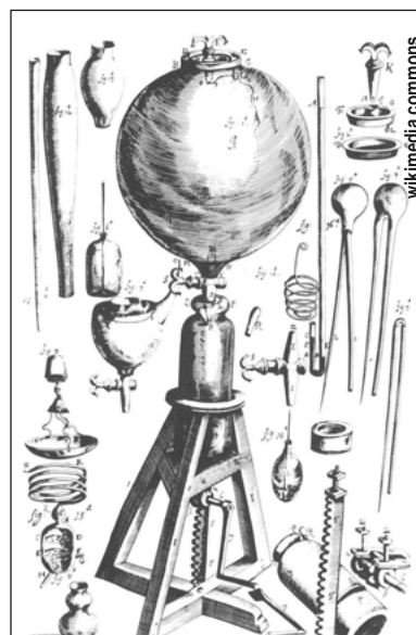
Engraving of Robert Boyle's "pneumatic engine" air pump and related instruments
