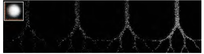
Four images of the vessel model. From left to right, particle concentration increases. CREDIT: Y. LI, O. AMILI, F. COLETTI / PR FLUIDS
