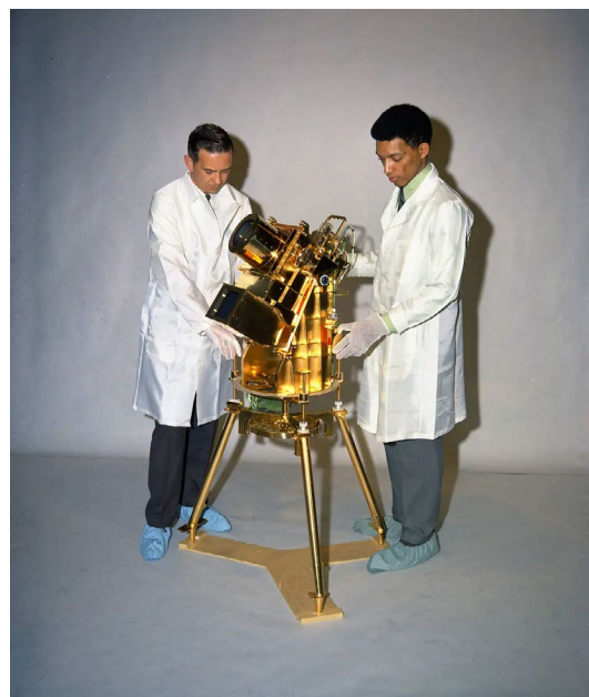
George Carruthers, right, and William Conway, a project manager at the Naval Research Institute, examine Carruthers' ultraviolet camera for the Apollo 16 mission to the moon. Credit: NASA
