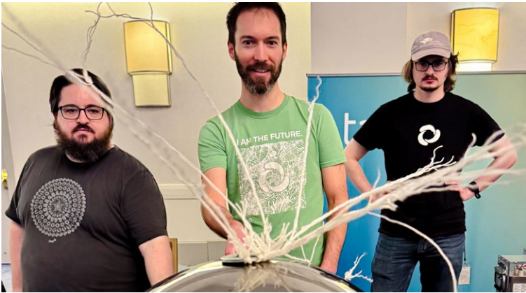
Three volunteers stand behind a Van de Graaff generator as it creates static electricity, causing the yarn on top to stand up. Credit: APS
