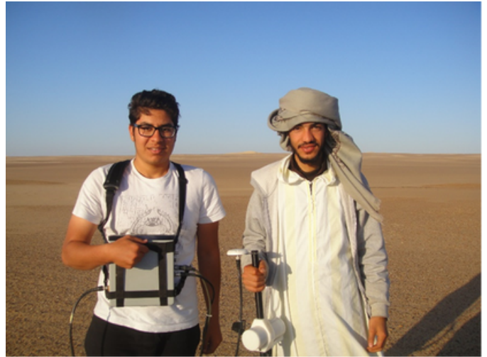
Figure 2: Measurement of the earth's magnetic field using the GEM magnetometer. (Photo Credit: The authors)
