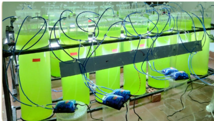
Figure 2: A photograph presenting an array of photobioreactors for biodiesel production of cultivated algae exposed to white light after being irradiated with a laser source. (Photo Credits: NA)
