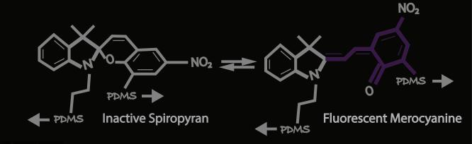
Here it shows a direct observation of damage in a mechanophore (MP) functionalized PDMS matrix due to localized stresses in the fiber-reinforced composite.
