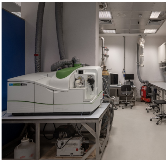
Figure 3: Overview of the Inductively Coupled Plasma Mass Spectrometer (ICP-MS) at the NMEC. (Photo Credit: NMEC)
