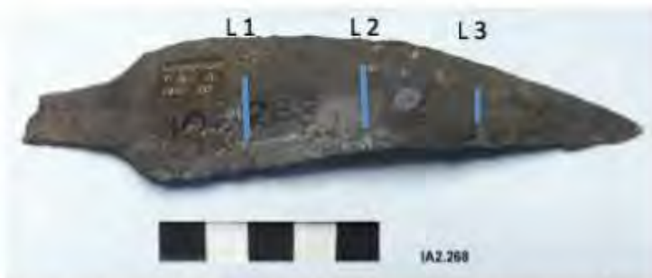
Approximate locations of the three positions used for residual stress measurements of IA 2.268.
