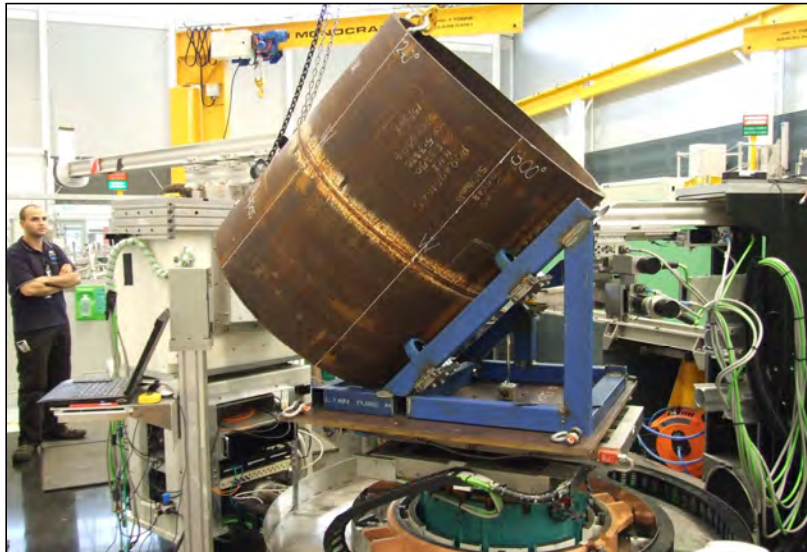
630kg pipe + supporting frame of ~200kg 1m diameter x 1m length x 28mm steel thickness
