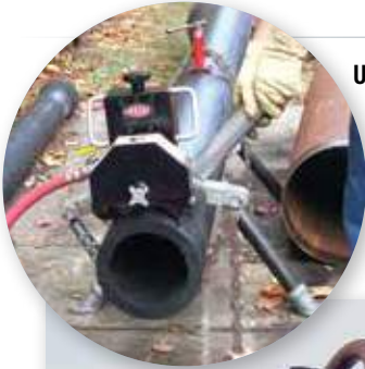
UPC636A on ductile iron
