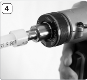
Expand the Tubing
