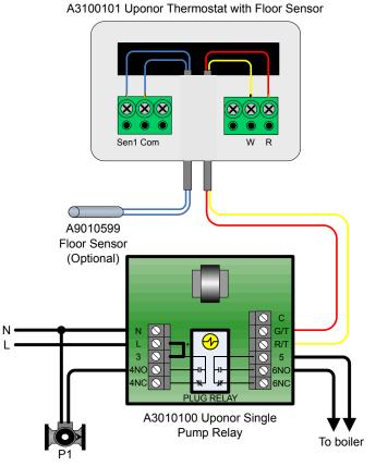
Figure 2: Uponor thermostat wired to a pump relay
