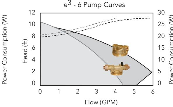
— UltraCirc Housing Flow      - - - - UltraCirc Housing Energy Consumption
