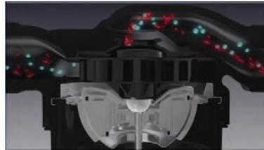
The main flow of the pumped media (blue) and its magnetite and sludge particles (red) flow outside the influence area of the permanent magnet rotor (bottom).
