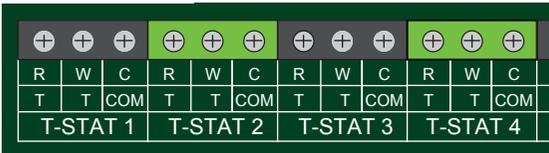
When a zone has a demand from a thermostat (T T / RW ) the control will send 120 VAC to the corresponding zone pump, primary pump and the (X X) dry contact will close to signal the boiler of a heating demand. AUX dry contact
