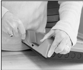
Insert screwdriver and push tab inward, cover should release from base.
