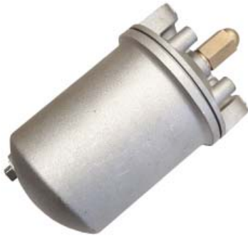
aluminum filter housing port sizes : 3/8", 125psi uses filter CUNO-300 or CUNO-300PT body diameter : 3-1/8" overall size : 3-5/8 x 6-1/2
