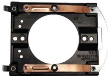
2 sets of contacts mounting holes : 2-3/4 & 3-3/8" c.-c. plate size : 3-7/8 x 3-1/4", hole I.D. : 2-1/4"
