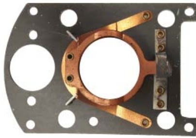
1 set of contacts mounting holes : 2-11/16 x 3-11/16" C.-C.
