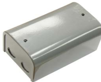
relay enclosure heavy gauge sheet metal four 1/2" knockouts size : 5-5/16 x 3-3/8 x 3-1/8" high
