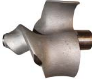
F-style 410 stainless steel impeller ref : 4353101, 10hp (492) chopper design 30mm bore x 181mm width x 205mm length
