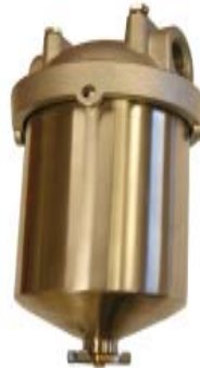
stainless Steel filter housing port sizes : 1/4", 300psi uses filter CUNO-300 or CUNO-300PT body diameter : 3-1/2" overall size : 4.20 x 7.50"
