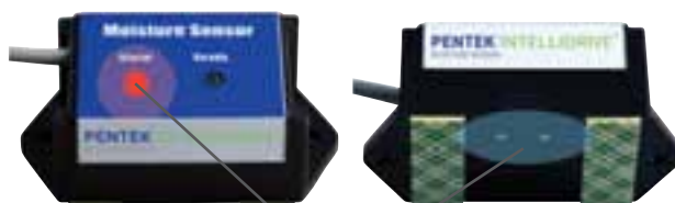
Fig. 2 Red "Alarm" Indicator is illuminated if water is touching the two detection points on the bottom of the Moisture Sensor.
