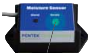
Fig. 1 Green "Ready" Indicator Illuminated
