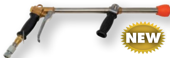
WG-GA-HD 850 psi 25 GPM heavy duty washdown gun with 1/2" male NPT swivel joint inlet and female coupling adapter
