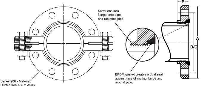
Ductile Iron ASTM A536 Grade 65-45-12
