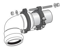
3. Insert extra long rod (provided) through bolt holes on the restrainer and through bolt holes on back-up ring. Place washers against restraint ring and back-up ring ears.
