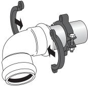
2. Install split back-up ring behind gasket race of fitting (make sure the bevel faces the gasket race). The two halves interlock at the bolt holes.
