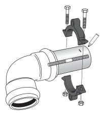
1. Install Series 1300 split restraint ring on the spigot end of the pipe. (Use connecting rod as a guide to position split restraint ring.) Tighten clamping bolts evenly at least to the minimum recommended torque. Install pipe into fitting.
