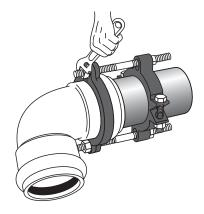
4. Tighten nuts behind back-up ring and restrainer. (Hand tight retaining nuts, then one revolution...do not over-tighten).
