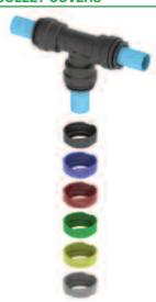
The slip-on Collet Cover shown in the illustration prevents accidental removal or tampering with tubing. Tubing can be inserted with the Collet Cover already attached to the fittings or the cover can slide into position afterwards. The cover is easily removed when required and comes in a variety of colours for colour coding.
