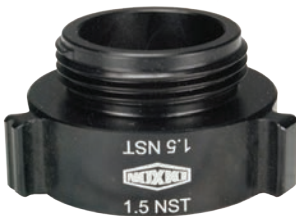
Extruded aluminum, anodized hard-coated with rocker lugs
