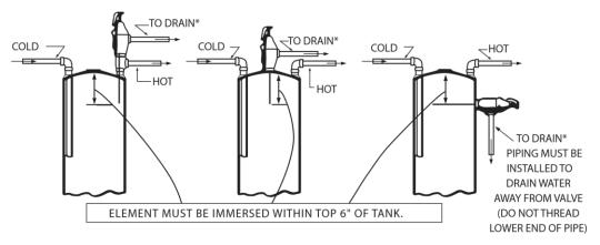
\* Piping to drain must be installed such that no point in the piping is higher than the relief valve and that there are no low points in the piping which will trap water.
