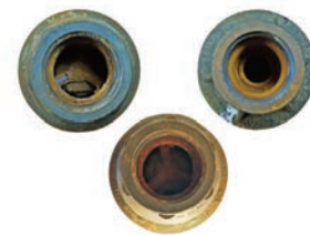
Inlet and outlet of worn pressure regulators.
