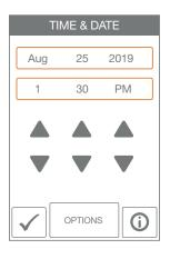
The time and date can be manually set by highlighting a field and then using the  ${\color{orange} \blacktriangle}$  or  ${\color{orange} \blacktriangledown}$  buttons.
