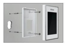
If the wall has damage extending beyond the width of the Thermostat, place the wall plate trim behind the back plate.
