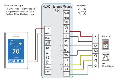
Up to 2-Stage Hydronic Boiler and 2-Stage Air Conditioner
