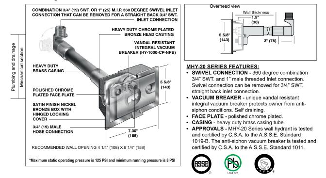
The wetted surface contacted by consumable water contains less than one quarter of one percent (0.25%) of lead by weight.
