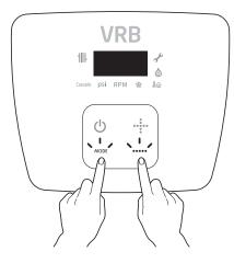
Press the MODE button to switch between the information types.
