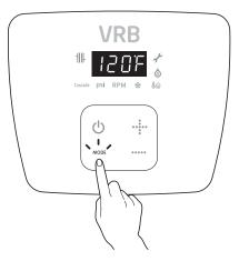
Press the ••• or •••• buttons until the desired temperature appears on the digital display.
