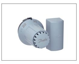
The flow temperature control (FTC) is used to regulate & maintain fluid temperature for hydronic floor or radiator heating systems. FTC is a self-acting thermostatic sensor, which can be combined with two-way valve body types
