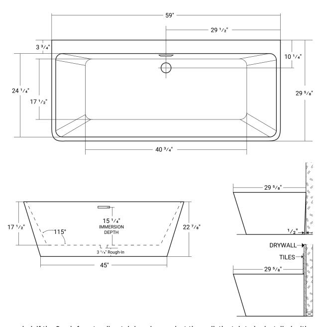
Recommended: if the Semi- freestanding tub is going against the wall, the tub to be installed with the supplied tiling flange.
