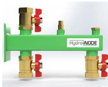
Wall bracket comes with 3 ball valves, 1/4" Manual Air Vent, and 1/4" NPT plug
