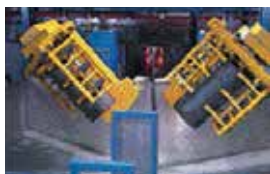
Once tanks are filled with PermaGlas, they are rotated (computer controlled) for precise, even coating.
