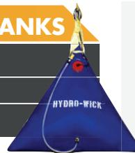
These aerodynamic Hydro-Wick® Fireflyers are used extensively by the forestry service to transport water, foam or potable water to remote locations by helicopter. The compact, flexible containers are made from a tough PVC coated fabric. Supplied complete with a 4"/102mm filler, shut-off at the outlet, standard GHT hose with "O" ring for attaching to harness clip and special pear shaped ring to resist rollout.
