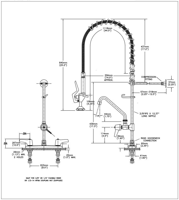
Delta reserves the right (1) to make changes to specifications and materials, and (2) to change or discontinue models, both without notice or obligation. Dimensions are for reference. Measurement may vary plus or minus 6mm(0.25"). Mounting locations are suggested only. Check with local codes for requirements in your area. This spec was produced September 18, 2017.
