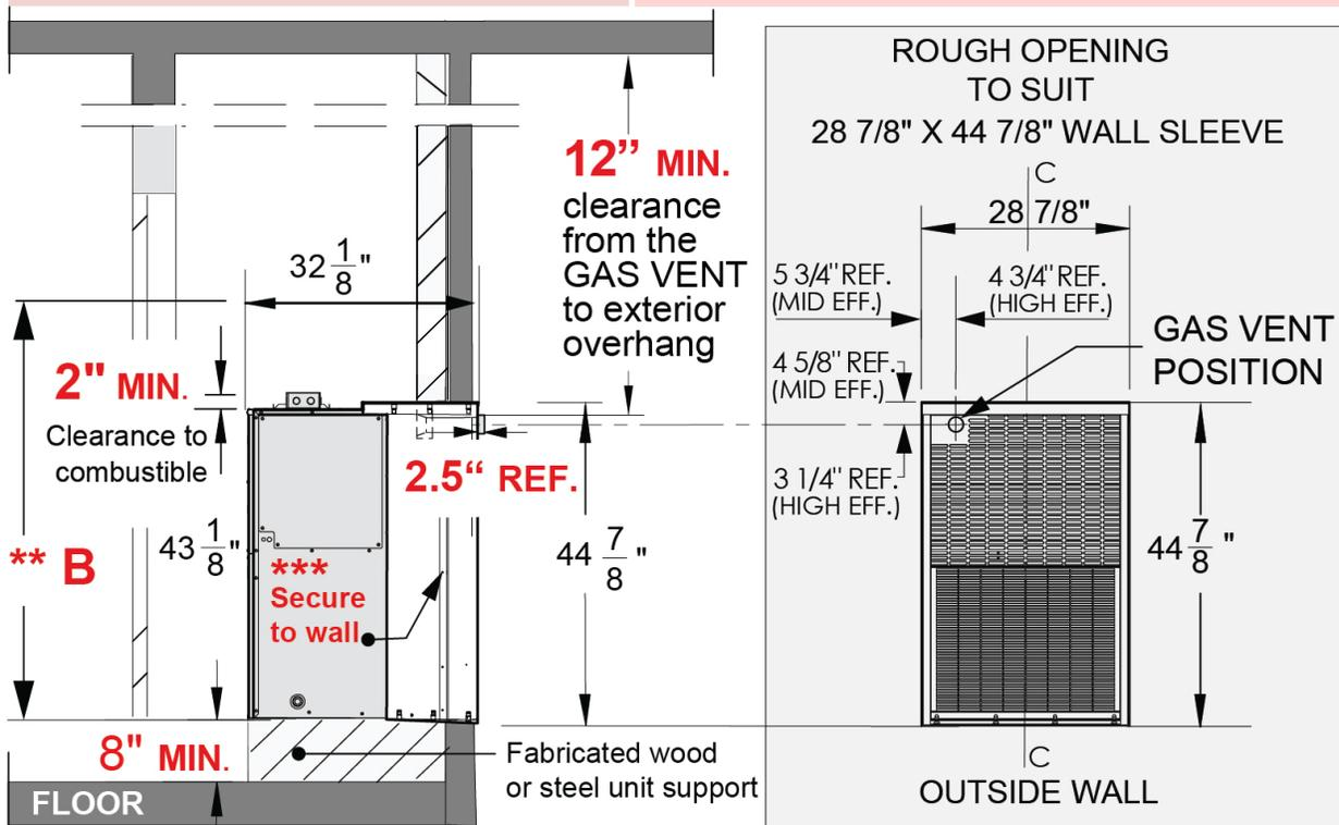
**IMPORTANT:** Minimum required vertical clearance of a vent terminal and overhanging structure from the top of the gas vent is 12" (more than 12" is recommended). Check local building codes for other requirements.
